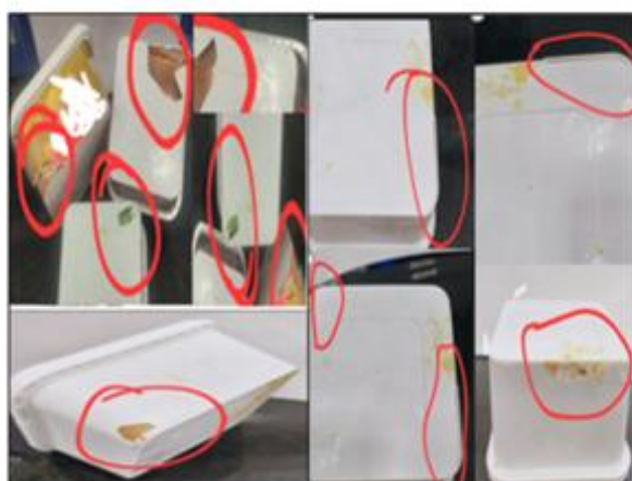
Figure 5. Product failure images after drop test (Trials 1–8). Red markings indicate observed cracks, breakage, and surface damage
