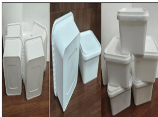
Figure 6. Product pass images after drop test (Trials 9–10). No visible cracks, breakage, or surface damage observed
