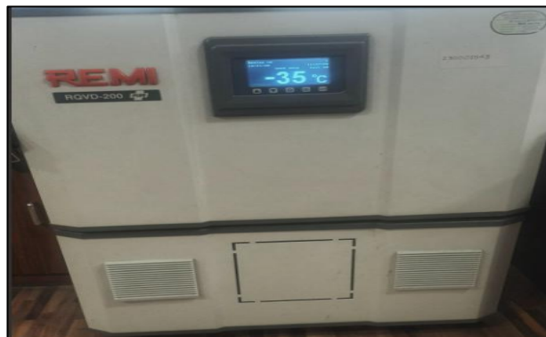
Figure 2. Deep-freeze cabinet (Remi RQVD-200 Plus) used for conditioning.
