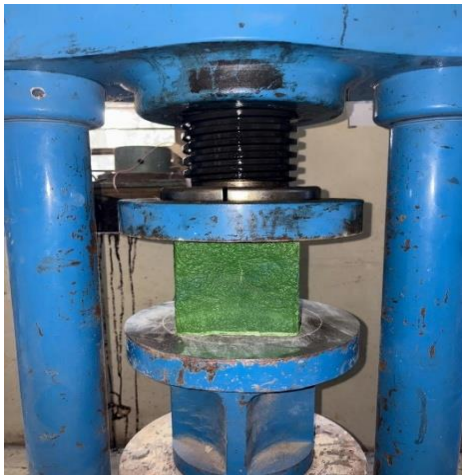
Fig 6: Recycled PP cube on UTM
