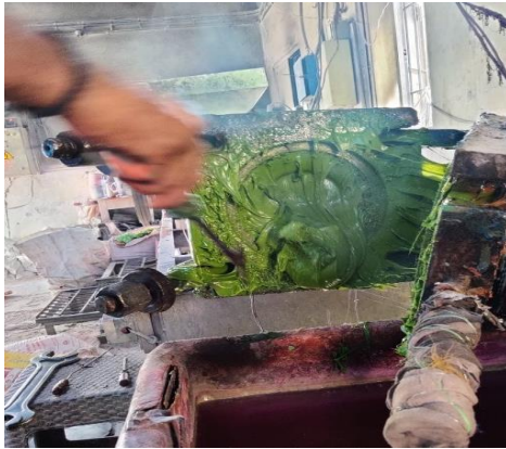
Fig 2: Collecting melted plastic from extruder
