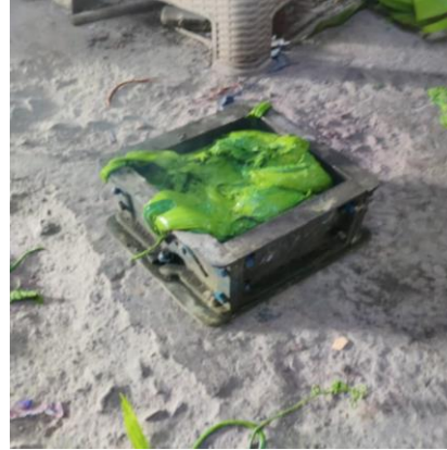
Fig 3: Pouring melted plastic into cube mould
