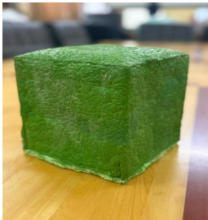
Fig 4: Recycled PP casted cube
