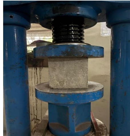
Fig 7: Concrete cube of UTM
