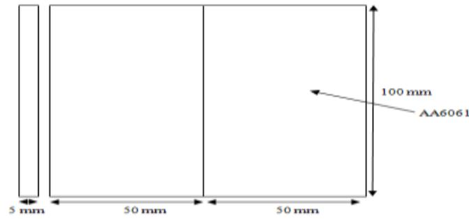
**Fig. 2 Square Butt Joint for Friction Stir Welding**
