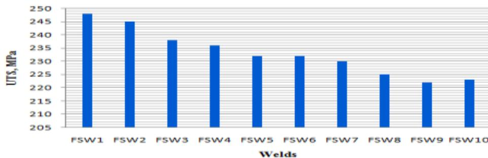
**Fig. 7 UTS for Different FSW Welds**
