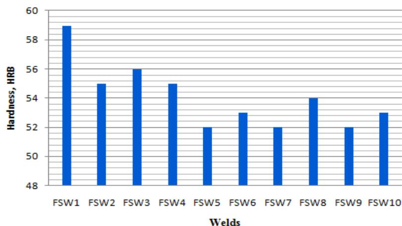
Fig. 6 Hardness Characteristics for Different FSW Welds
