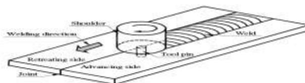
**Fig. 1 FSW Process**
