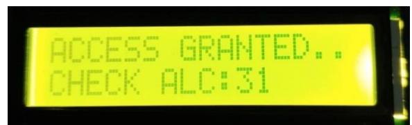
Fig 9 Checking alcohol and access granted
