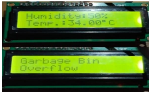
Fig. 3: Display Status of Humidity, Temperature and Garbage
