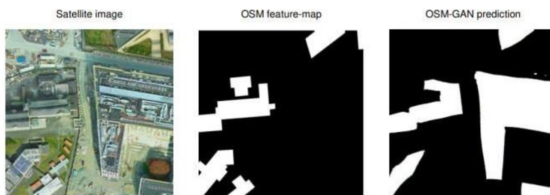
Figure 4: The OSM-GAN prediction detects building object changes in a satellite image
