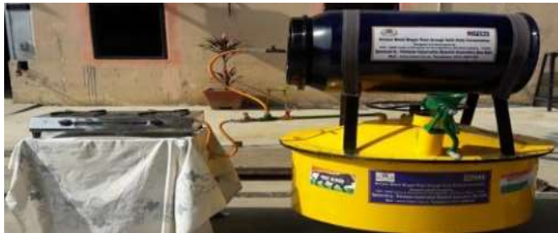
Fig -2: Anaerobic digester
