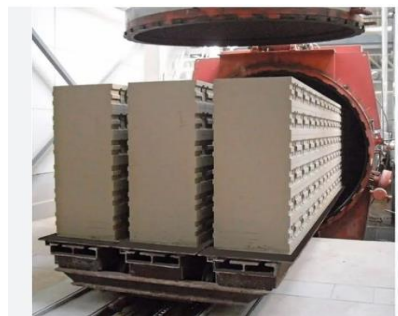
Fig 2: Steam Curing Chamber
