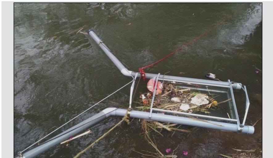
Fig. 1 Litter trap in river
