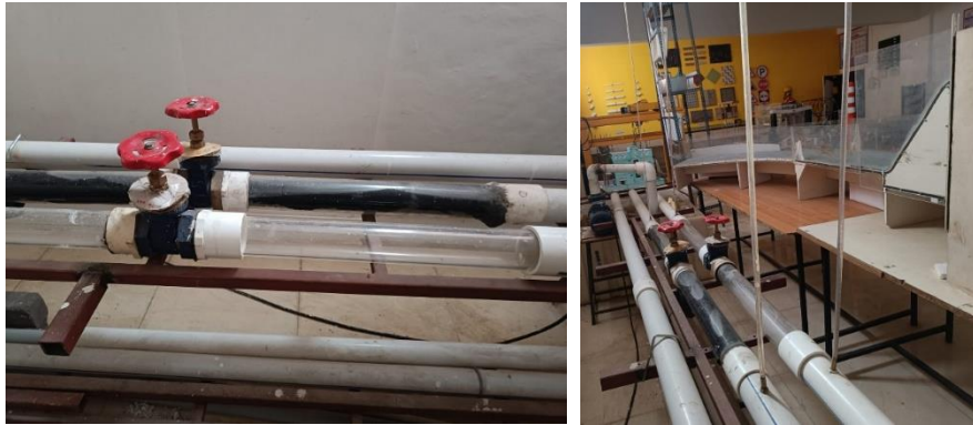
Figure 2: Experimental setup (a) with and without rubber sleeve and (b) piezometer at both end of valve
