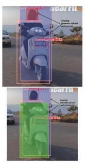
Fig3.b Checking Overlap between person and motorcycle Method 1
