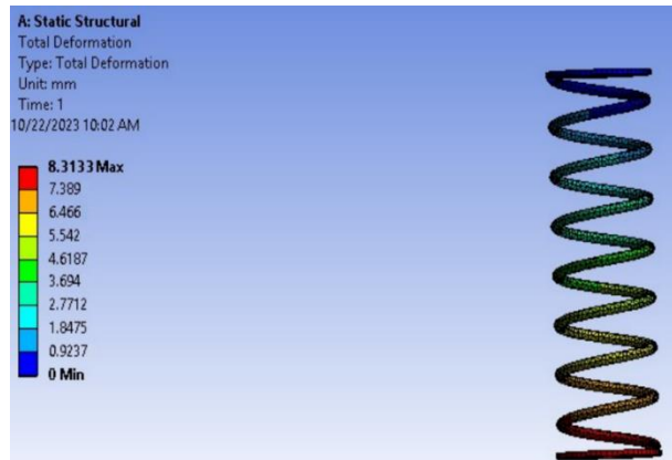
Fig. 3.Total Deformation for Structural Steel at 100N Load
