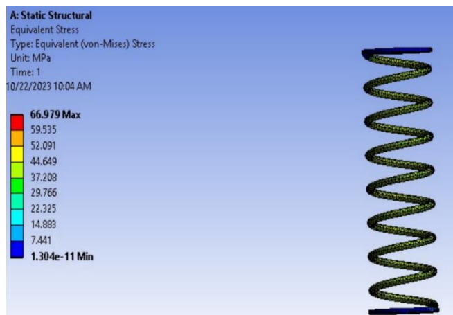
Fig. 4. Von-Mises Stress for Structural Steel at 100N Load
