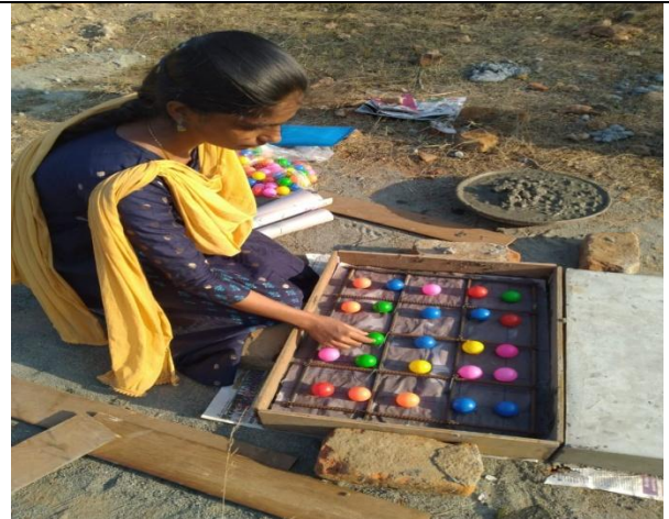
Fig. 3.3 Insertion of plastic balls (25) in slab casting
