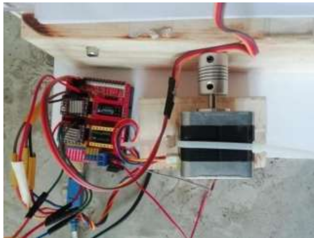
Figure (6): CNC shield board and a4988 motor driver
