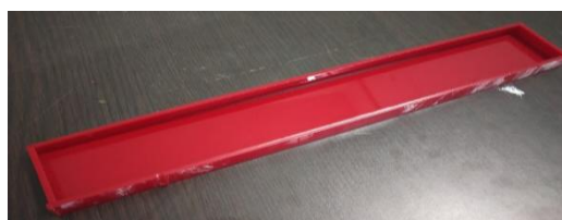
Fig 3. Mould for composite fabrication
