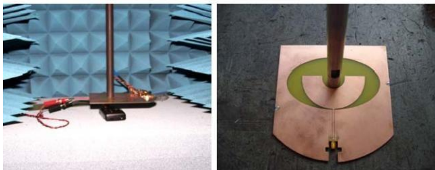
Fig. 7. Detecting antenna with EMC testing unit developed at Queen Mary, University of London
