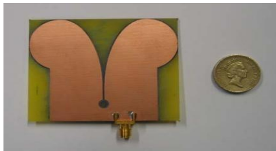
Fig. 2 Vivaldi antenna configuration for impulse radar applications
