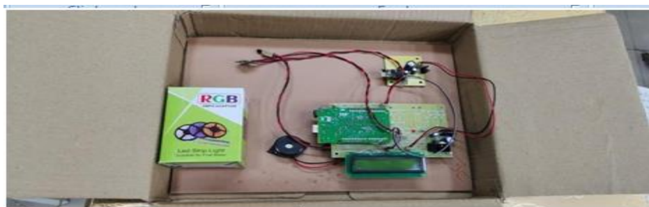
Figure 6: Patient monitoring and alert system kit
