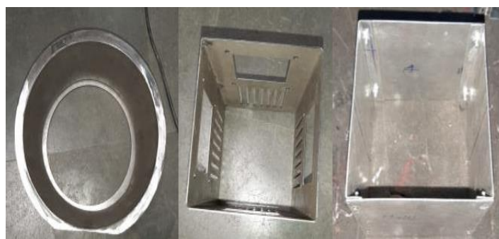
Fig-10: Hoop, Main Base, Aluminum Box after sheet metal cutting
