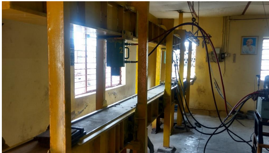
fig.1 static bending strength test of sleepers
