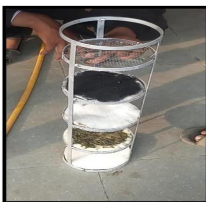
Fig 3.4 Image of Filter Unit
