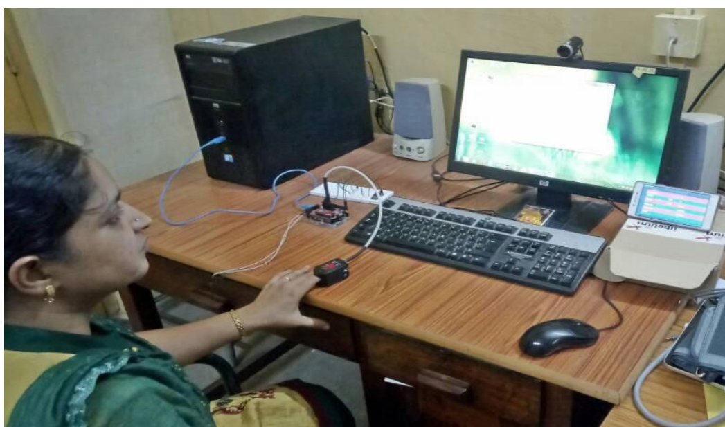
Picture1: Setup of pulseoxy measurement for wireless Telemedicine system
