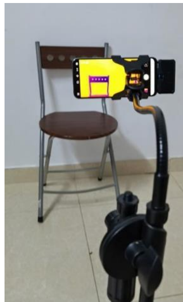
Figure 2: Examination room thermal camera with one-meter distance from the chair
