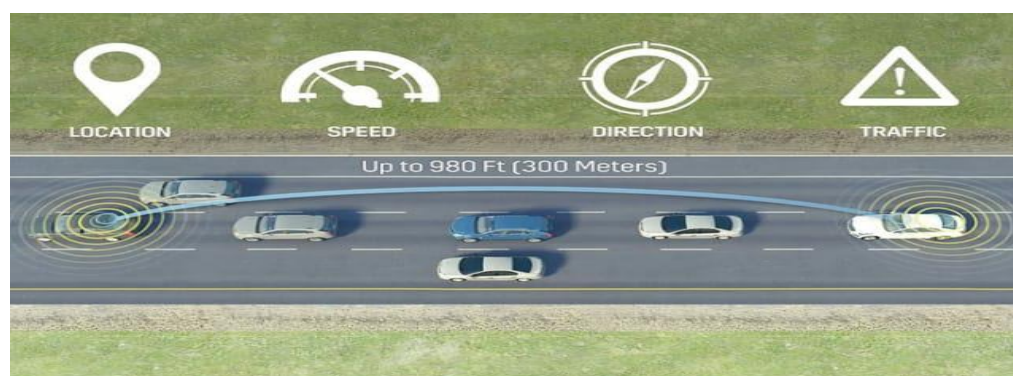
Fig : 4 Vehicle to Vehicle Signal Transmission
