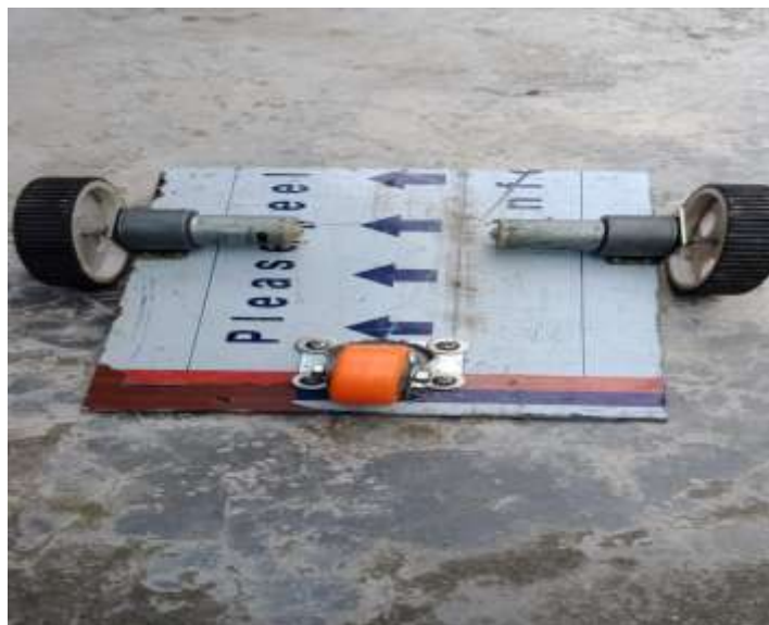
Fig-4.4:Base assembly of the robot (bottom side)
