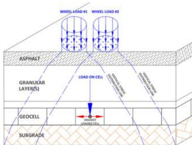
We can see at the pic above that part of any vertical load on any of the cells is transferred to lateral load turning to hoop stress on the cell wall.
