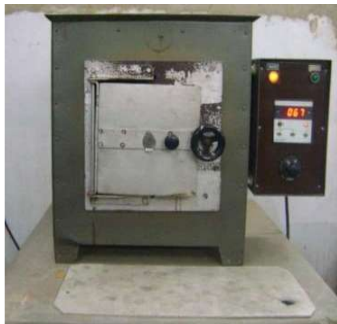
Fig 3.5(c) Muffle furnace
