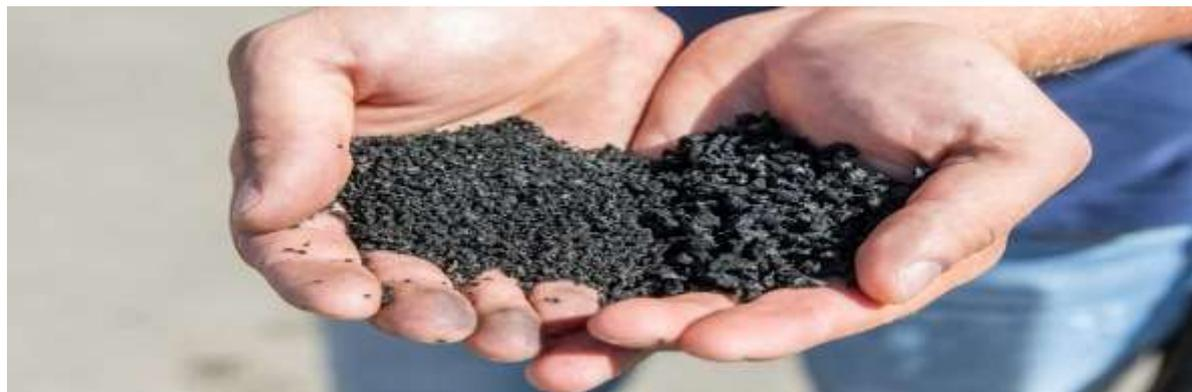
The use of waste tyres in construction of roads brings out a better performance. There is better binding of bitumen with waste tyres. The frequency of voids is also reduced due to increased bonding and area of contact between polymers and bitumen.
