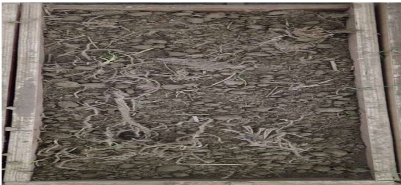
(Field 2-Field using crushed jute and jute used in upeer layer)Fig
