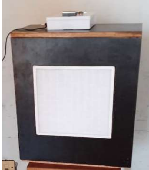
Figure 5: Hardware System of IOT based Air Purifier with Pollution Monitoring System
