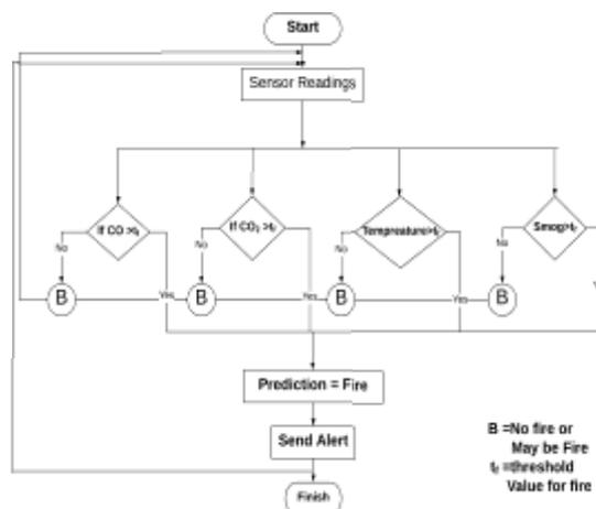
Where **t1** is the threshold value of the fire and **B** is the no fire.
