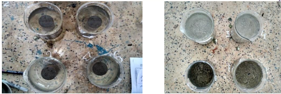
Fig 3.6: Wet Dry test sample before and after failure.
