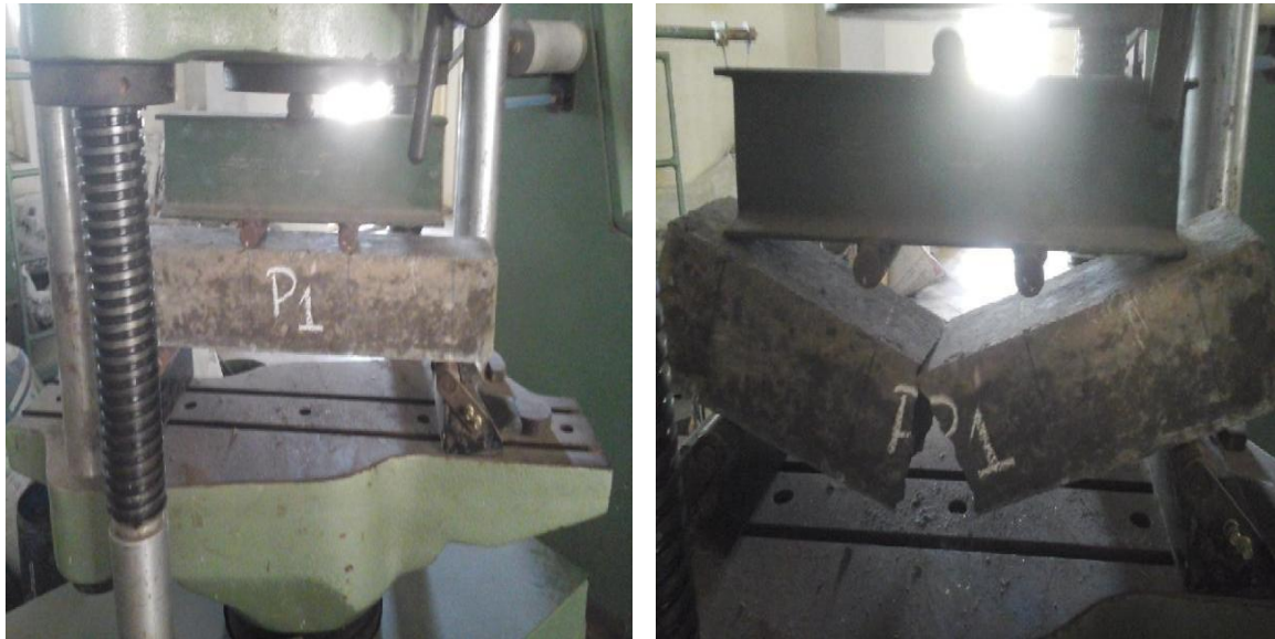
Fig – testing of specimens for flexure strength
