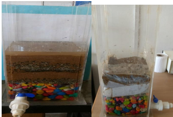
1. Slow sand filter 2. Rapid sand filter
