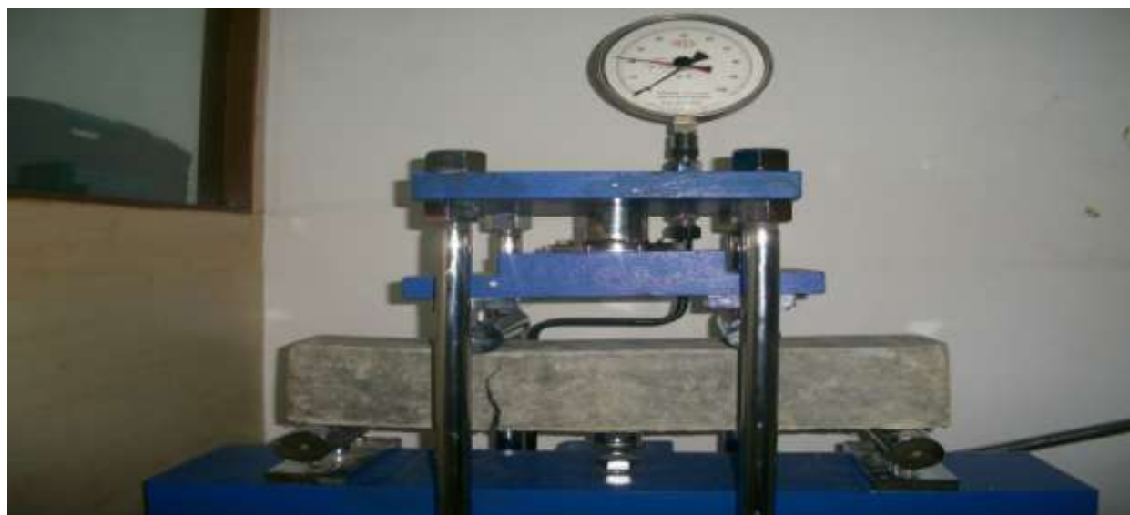
Figure 5.6: Flexural strength test of beam
