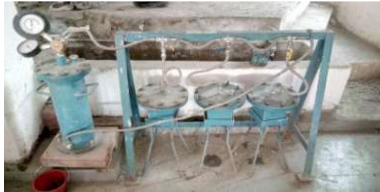
Fig.7 Permeability Test Apparatus
