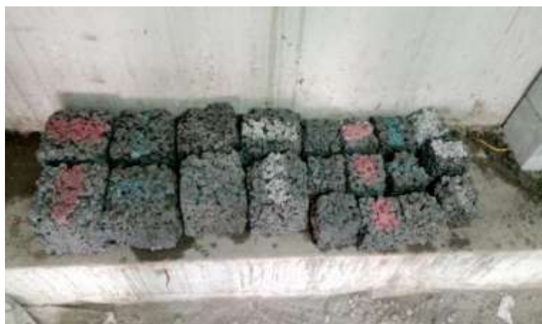
Fig.3 Test Specimens for compression & Permeability Test
