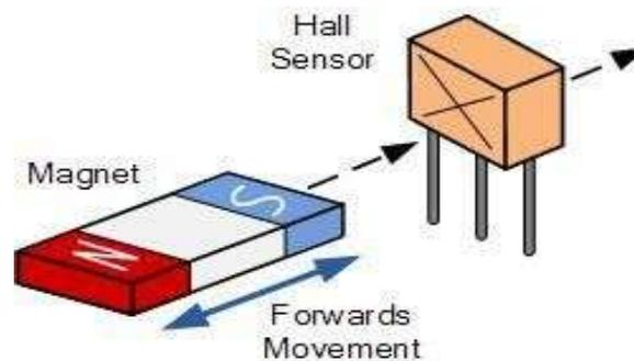
Fig 6.Head on detection.
