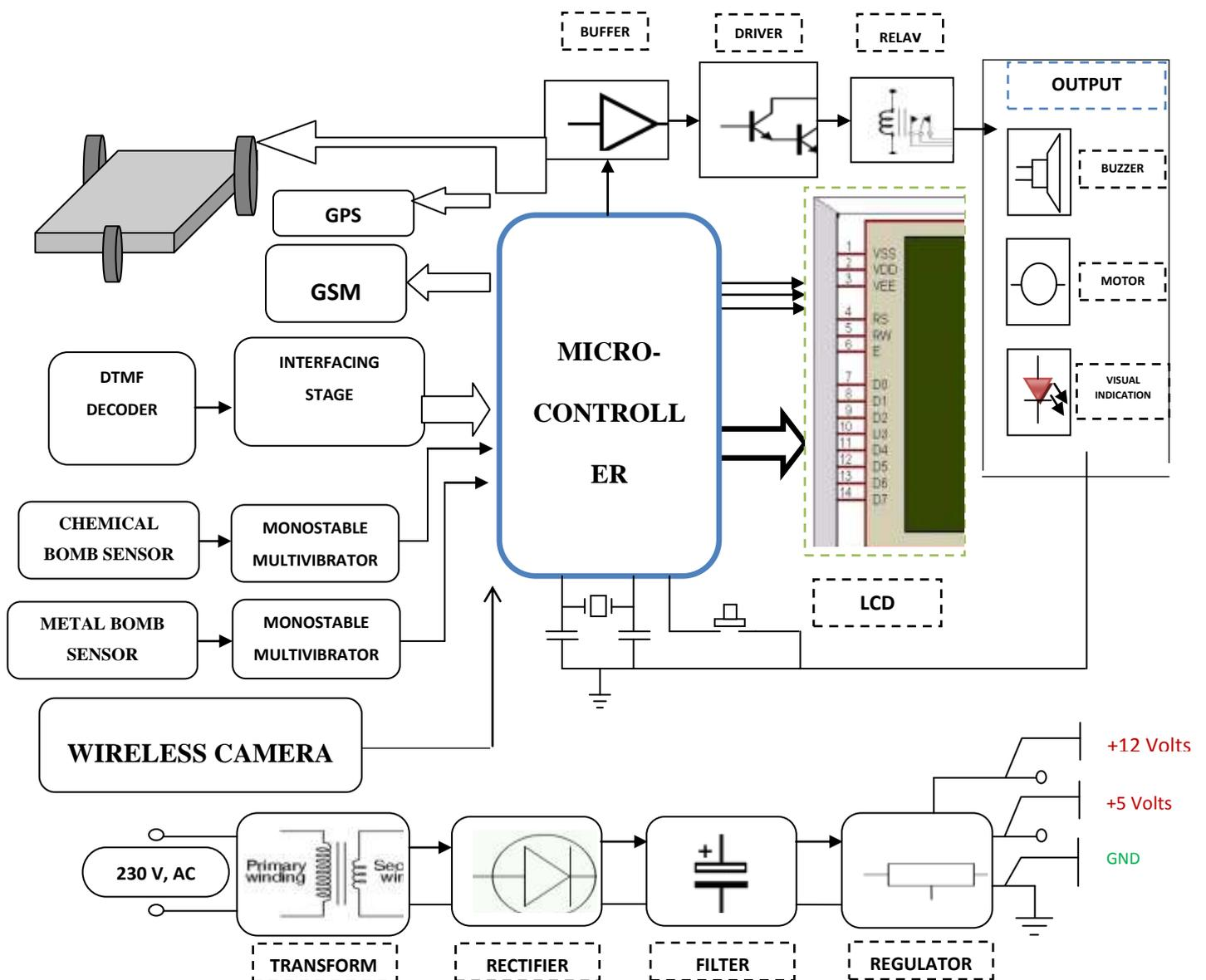
Fig 1. Block Diagram of Land Rover Robot.
