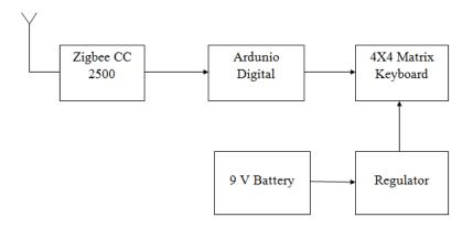
Fig 2: Block Diagram oftransmitter of greenhouse surveillance
