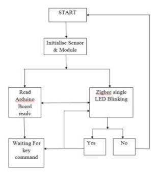
Fig.4Transmitter work flow
