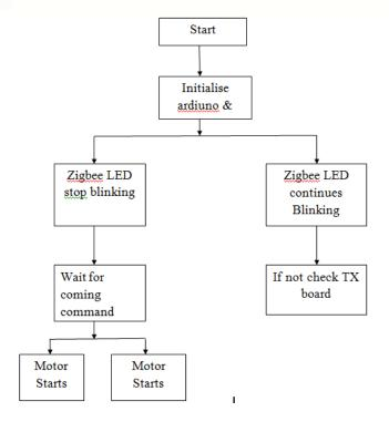
Fig.4 Receiver work flow
