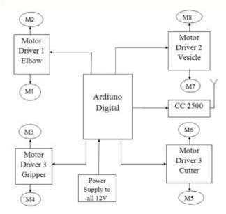
Fig 1: Block Diagram ofreceiver of greenhouse system
