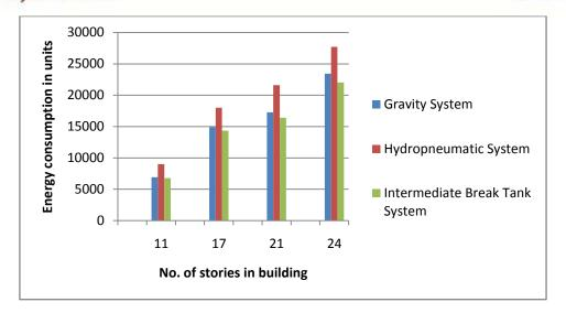
The above two table and graph shows that the energy consumption profile for intermediate tank system is less than gravity and hydropneumatic pressured system. From these tables it is clear that energy consumption profile of intermediate system is less than two systems so it is necessary to carry out the detailed overall cost analysis of three systems to get clear picture.
