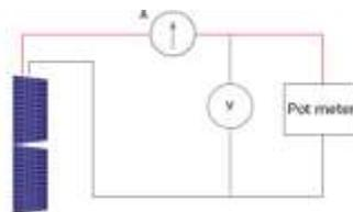
Fig. 4(a) Circuit diagram for evaluation of I-V and P-V characteristics of series connected modules
