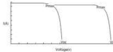
Fig. 3(a) I-V characteristic of series connected modules
