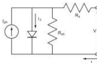
**Fig. 2 Equivalent Circuit of Solar PV Cell**
