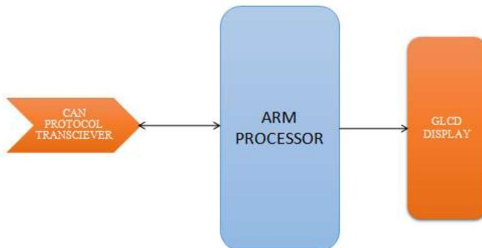
Fig.2. Receiver section of the proposed system.
