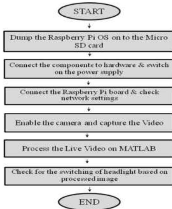
Fig.2. Flow diagram of software setup
