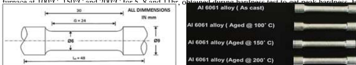
Figure 2: Sample prepared for Ultimate tensile strength test (ASTM-E10M)
