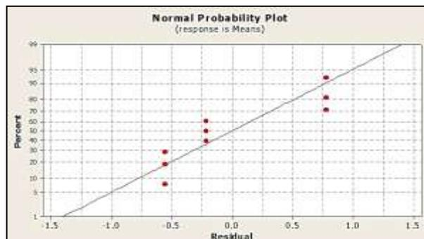
Figure 6: Normal probability plot for UTS measurement.
