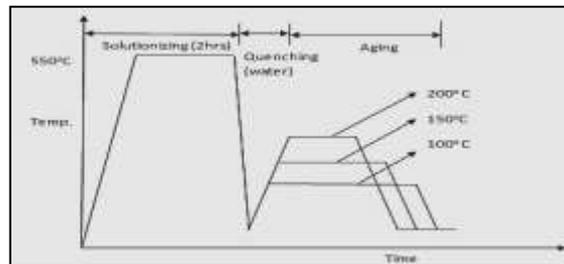
**Figure 3: Age hardening treatment cycle for Al 6061 alloy**
