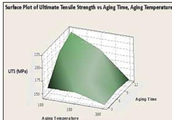
Figure 5: Surface lot of UTS vs aging time and aging Temperature
