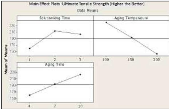
Figure 4: Main effect plot of UTS for the age hardening of Al 6061 alloy
