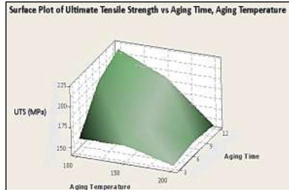
Figure 5: Surface lot of UTS vs aging time and aging Temperature
