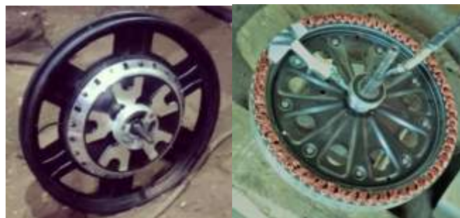
Fig. 2, BLDC Hub Motor And Winding Of Motor
