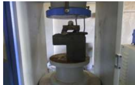
Fig 5 Experimental set up for shear test
