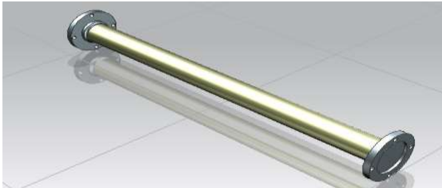
Fig.8 Design Of Composite Carbon Fiber Shaft
