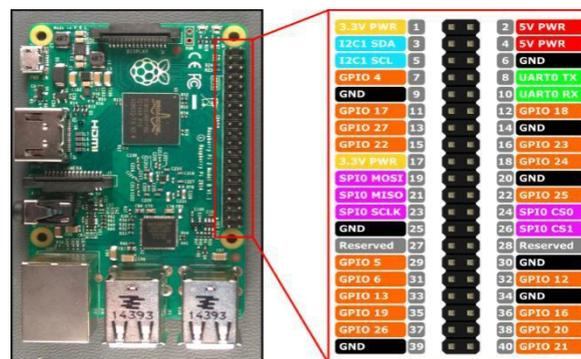
Fig 3.8.2 Raspberry pi 3-pin diagram
