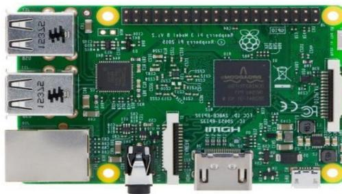
Fig 3.8 Raspberry pi 3 model B
