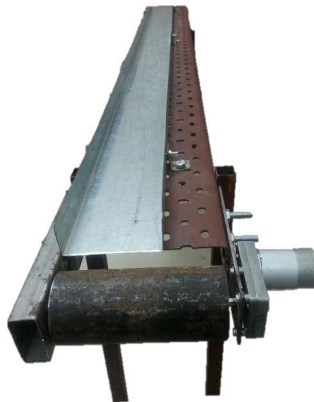
Fig. 6 DC motor connection to the conveyor system
