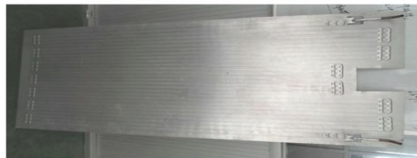
Fig 13. Representation of roll-bond heat exchanger
