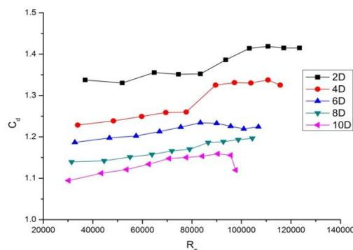
Fig 6:  $C_d$  v/s  $R_e$  at different upstream lengths for  $\beta=0.4$
