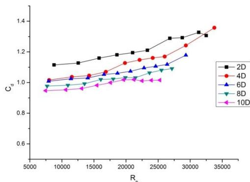
Fig 4:  $C_d$  v/s  $R_e$  at different upstream lengths for  $\beta=0.2$
