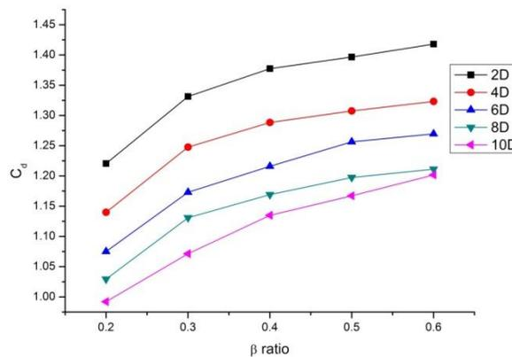
Fig 9: C<sub>d</sub> v/s β at different upstream lengths
