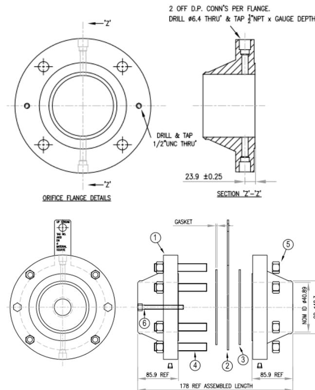
Fig 3: Section views of flanges and orifice
