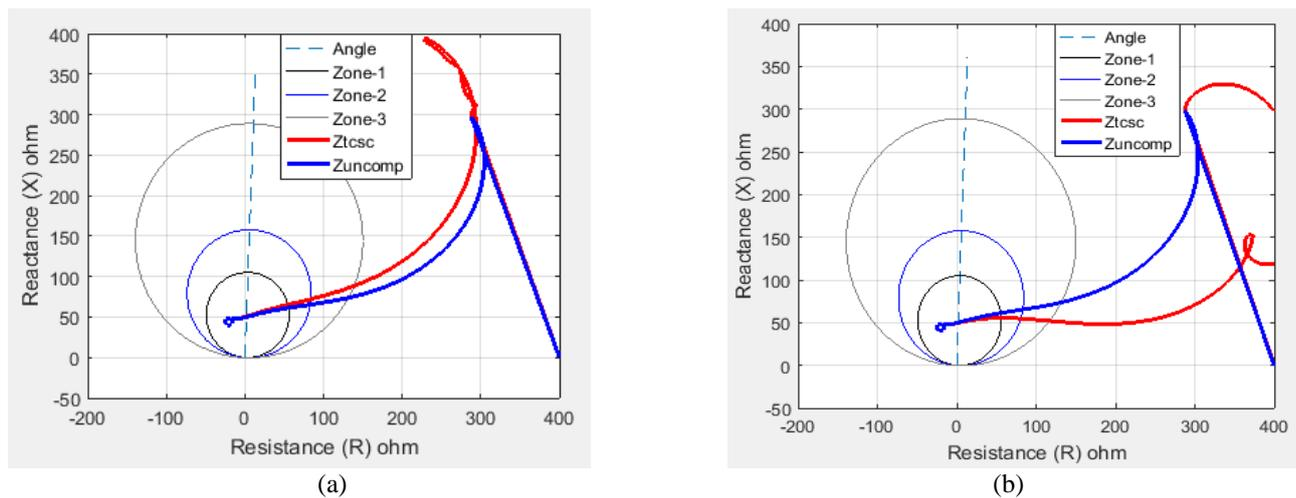
Fig. 5. Simulation results of at 150km LG Fault in compensated & uncompensated line; (a) Simulation results of  $\alpha=25^\circ$  at 150km LG Fault (Inductive mode) (b) Simulation results of  $\alpha=85^\circ$  at 150km LG Fault (Capacitive mode)
