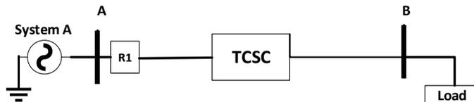
Fig. 3. Transmission line with TCSC in mid-point.
