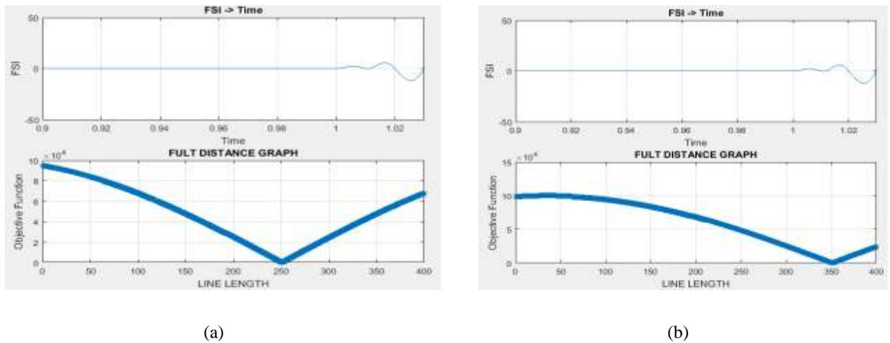
Fig. 9. Simulation results of algorithm for after TCSC different fault location at  $\alpha=25^\circ$ ,  $R_f=10\Omega$  LG fault
