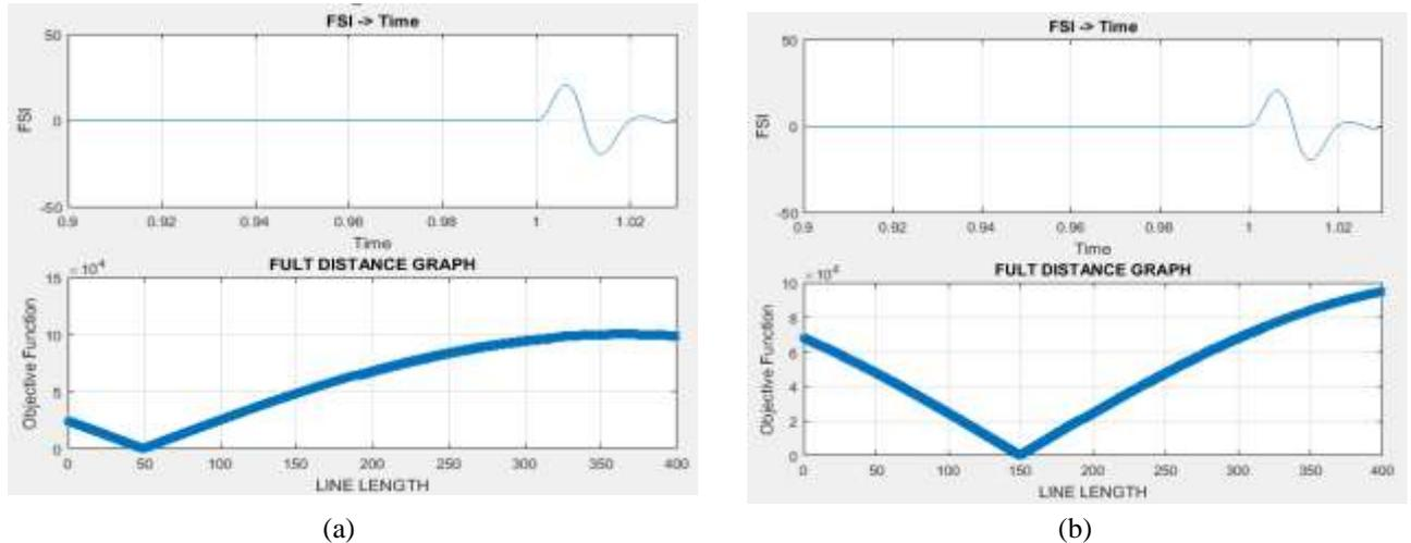
Fig. 8. Simulation results of algorithm for before TCSC different fault location at  $\alpha=25^\circ$ ,  $R_f=10\Omega$  LG
