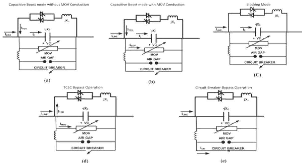
Fig. 2. TCSC operating modes during condition of fault.
